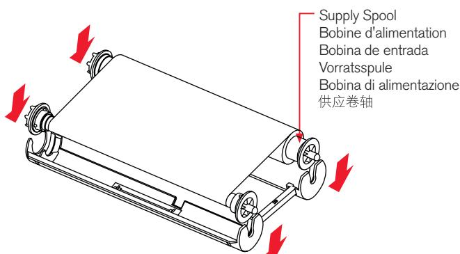
Using the handle, slide the spools onto the two hubs on the left side until they can engage the two holders on the right.
